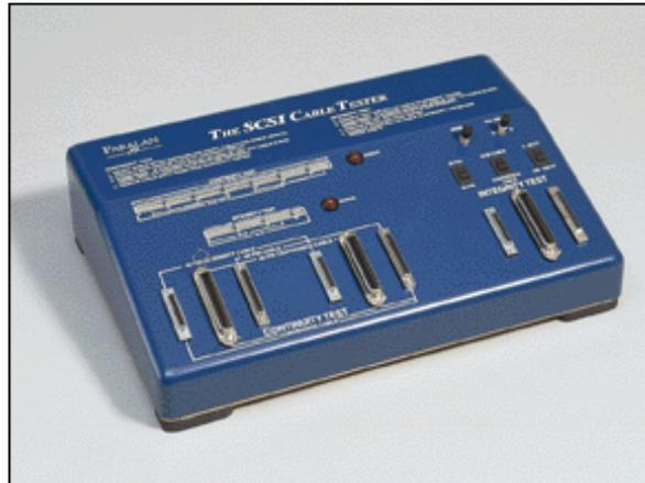
**The SCSI Cable Tester is designed specifically to test cable assemblies made to SCSI specifications!**
