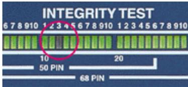
(Darkened indicator for twisted pair no. 13 shows Integrity Test failure)
