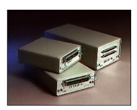
Now when your SCSI bus is just a bit too short, there is a simple, economical solution: a SCSI HVD expander, the Paralan RegeneratoR™. The RegeneratoR™ sends and receives SCSI transmissions at maximum sustained HVD SCSI data rate - up to 40 Mbytes/sec Ultra SCSI.
